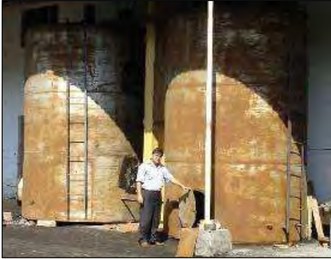
Proud owner showing off his newly constructed drying tanks from durable scrap metal left from Soviet era
