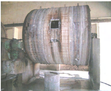
Drums for soaking and liming skins
