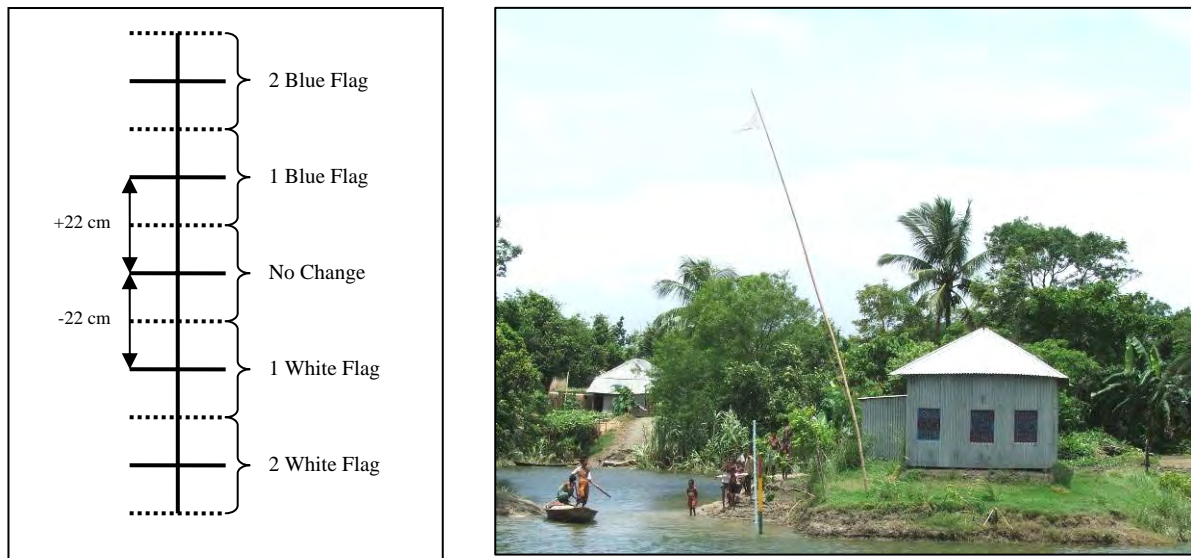
Figure 4.11: Schematic of Flag System, and a flag system in operation in the floodplain
