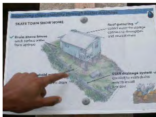
Above: A public awareness brochure of a “model home” retrofitted by the community as part of the PRF/MoSSaiC project. It explains proper installation of roof guttering and drainage pipes leading to the “STAR drains” and main drains.
