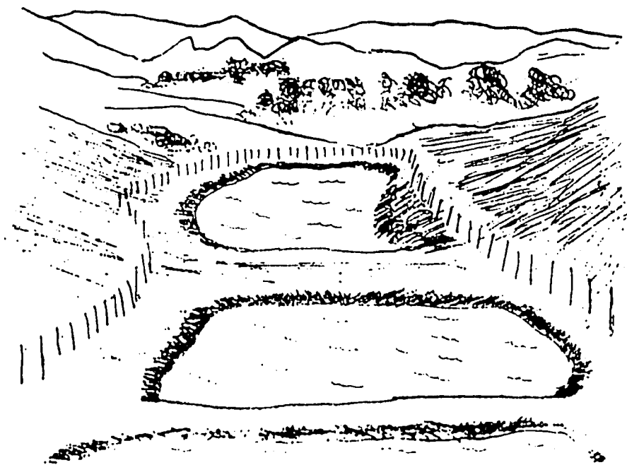
Figure 7: Small ponds provide opportunities for agricultural diversification. They are suitable for harvesting runoff water in rural areas, thus storing it for many purposes which include small scale irrigation, household uses, livestock watering and aquaculture. Ponds properly built and maintained have an indefinite life.
