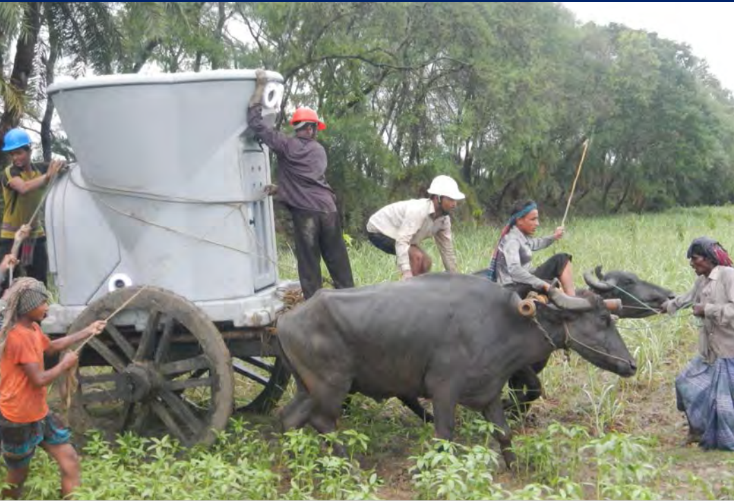
Transporting Sonic Detection and Ranging (SODAR) device for remote wind measurement in Bangladesh.
