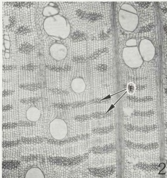
Figure 2.--Cross section (30X) of Erythrina subumbrans , from Philippines, with broad bands of axial parenchyma. Fibers (F) show as darker patches.
