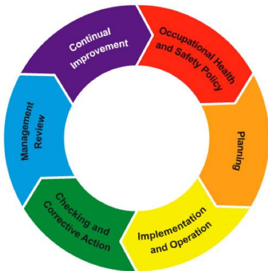
FIGURE 9.1: HEALTH AND SAFETY MANAGEMENT SYSTEM
