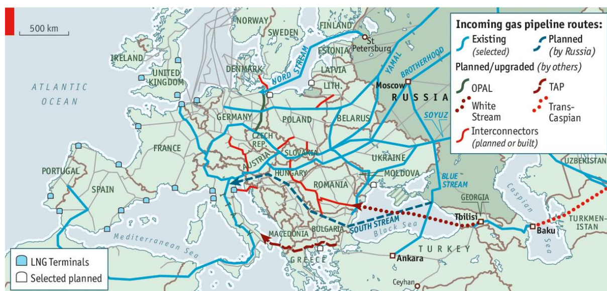
FIGURE 2.5: MAJOR EUROPEAN GAS PIPELINES
