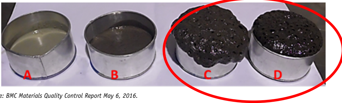
Figure 2 Thickening of abrasive slurry due to excessive amount of percentage fines
