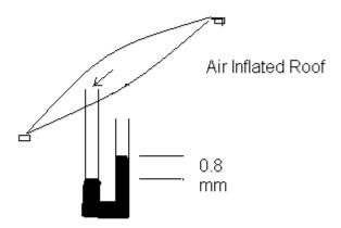
Air pressure changes length of water column. Adjust to 0.8 mm difference.
