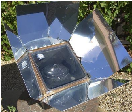
Figure 4: A solar oven
