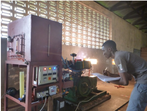
During training, a Biomass Brother runs tests and records data on the 5kW Lister Engine running on crude palm oil (CPO)
