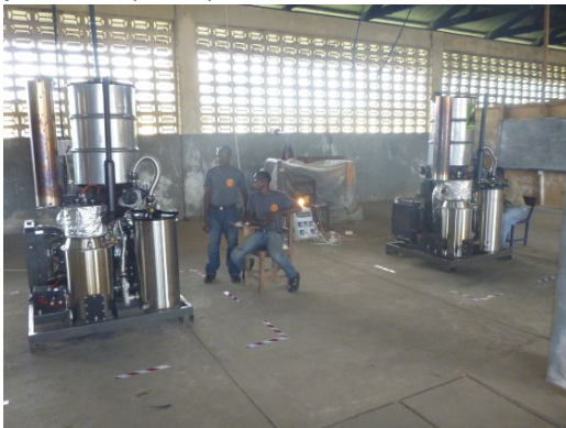
The Biomass Brothers operate BWI's biomass gasifiers using palm kernel shells as fuel
