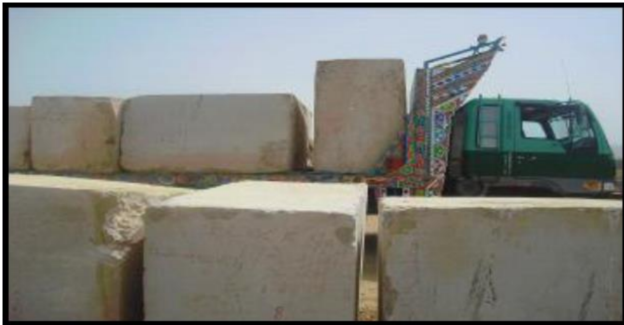
Figure 6 Transportation of Block Extracted Through Wire Saw
