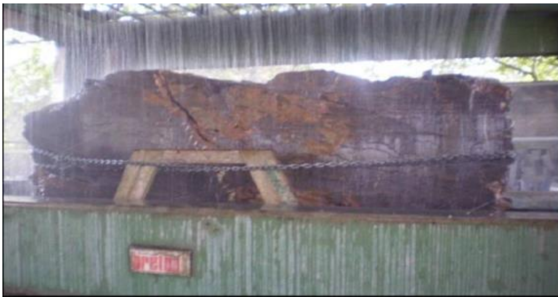
Figure 19 Highly Fractured Material under a Gang Saw
