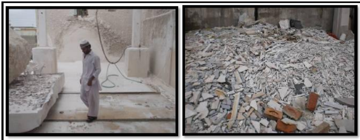
Figure 23 Poor Housekeeping at the Processing Plants
