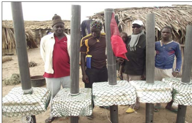
Figure 6. Constructed Spar buoys ready for deployment
