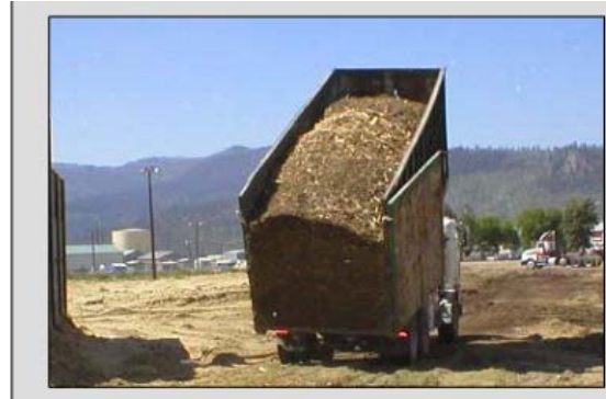
Hook Track Unloading Container
