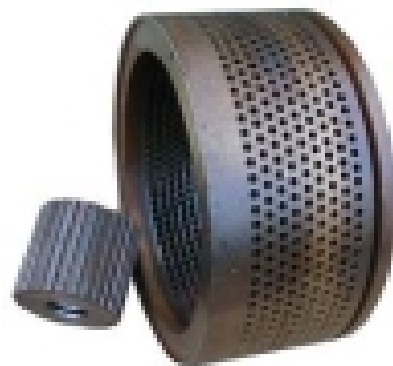
Figure 9.3. Key parts of pellet machine (roller and die)
