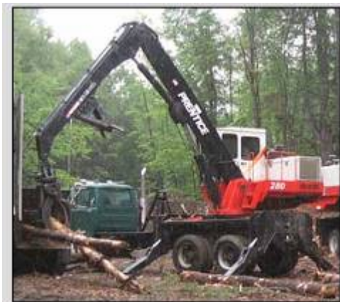
Photo 7.9 Loader on a Crane Carrier
