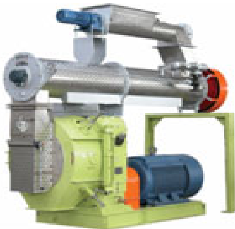
Figure 9.2. Example of small pellet machine (300kg/hour)
